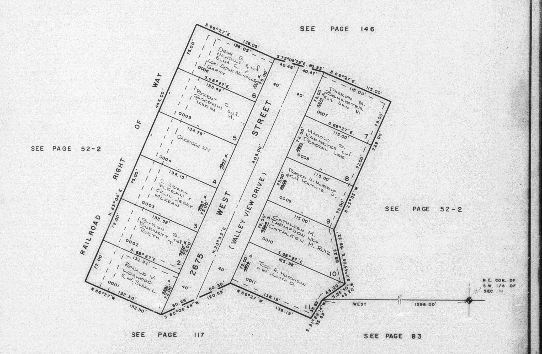
7' UTILITY & DRAINAGE EASEMENTS FACH SIDE OF PROPERTY LINES AS INDICATED BY DASHED LINES
